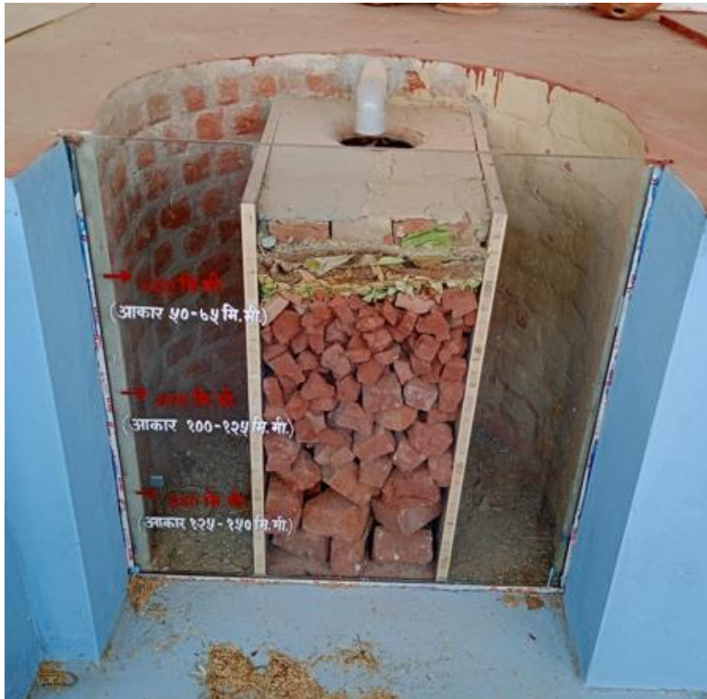
Household Soak Pit 1 m (depth) x 1 m (diameter)
