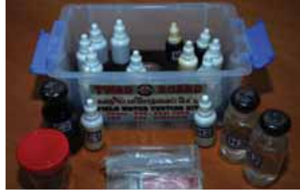
A kit for assessing water quality at the field level developed by Tamil Nadu Water Supply and Drainage Board
