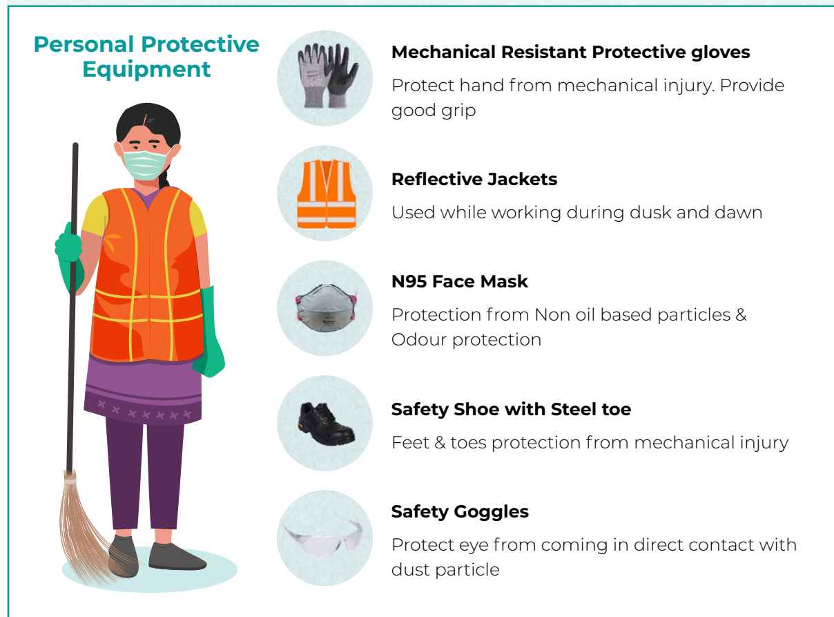
Figure 2: PPEs, Tools and Equipment required for street sweepers and door to door waste collectors
