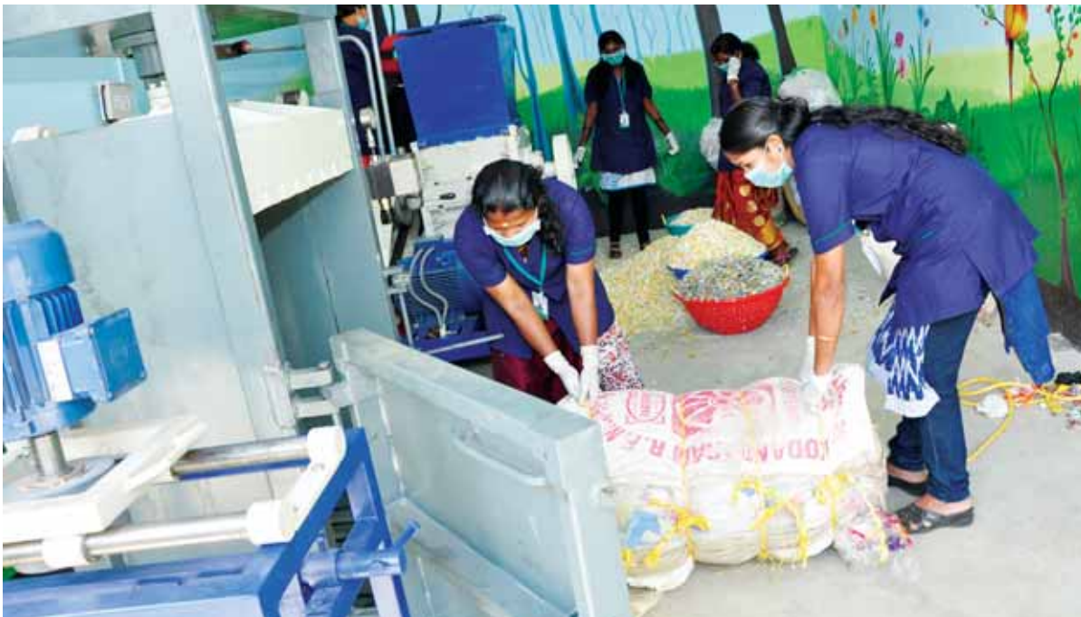
(From left to right) Plastic baler; plastic waste being baled, ready bales of plastic stacked
