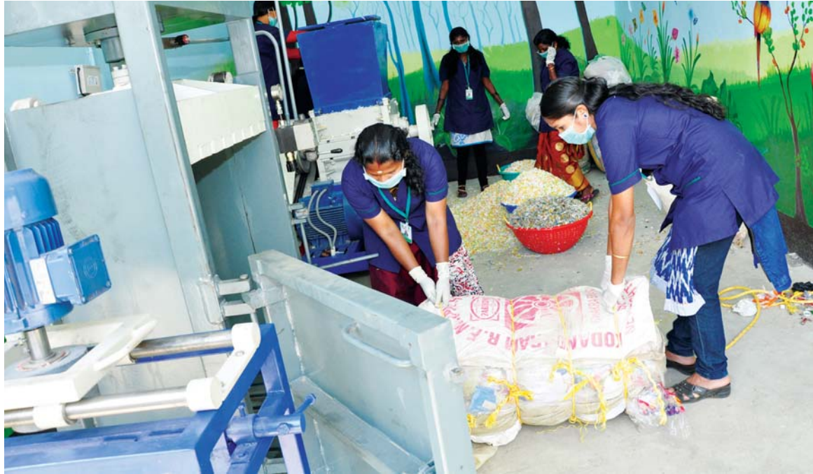
Figure 10: (From left to right) Plastic baler; plastic waste being baled, ready bales of plastic stacked
