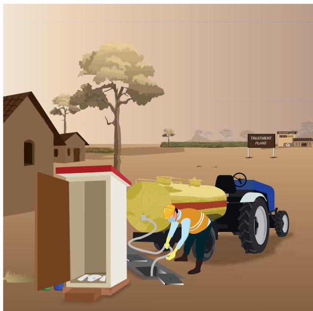
Figure 2: Single pit and septic tanks in full condition
