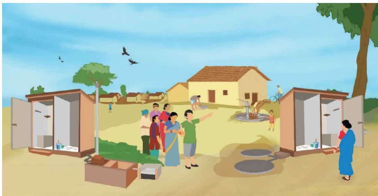
Illustration showing safe distance of drinking water source and twin pit toilet, septic tank toilet with soak pit for safe disposal of effluent
